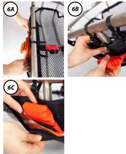
Figure 6 - Placing the sail in the pocket
