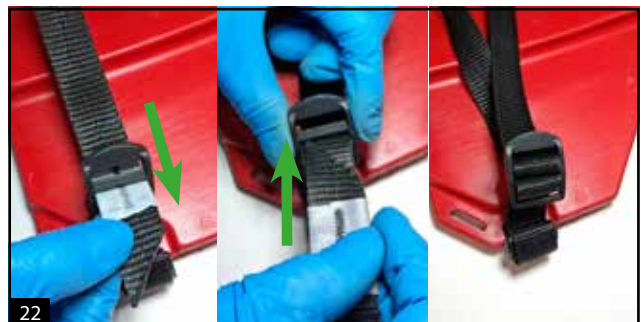
Securing the T-shaped band strap
