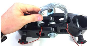
Pass the steel cable around the centre pin connecting the bipod head.
