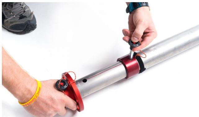
Lock the leg - extractable element - on the hole and insert the locking pin.
