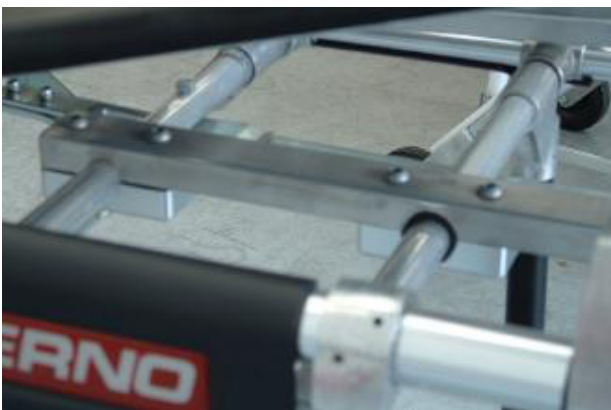
Figure 10 - Detail showing the front and central clamps.
